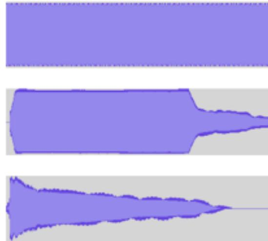
**Figure 1.** These are waveforms of a 1.5 second note played at 440 Hz. The first was made by a computer, the second by a saxophone, and the third by a piano.
